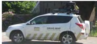
DRIVE-MAP Mobile mapping system
