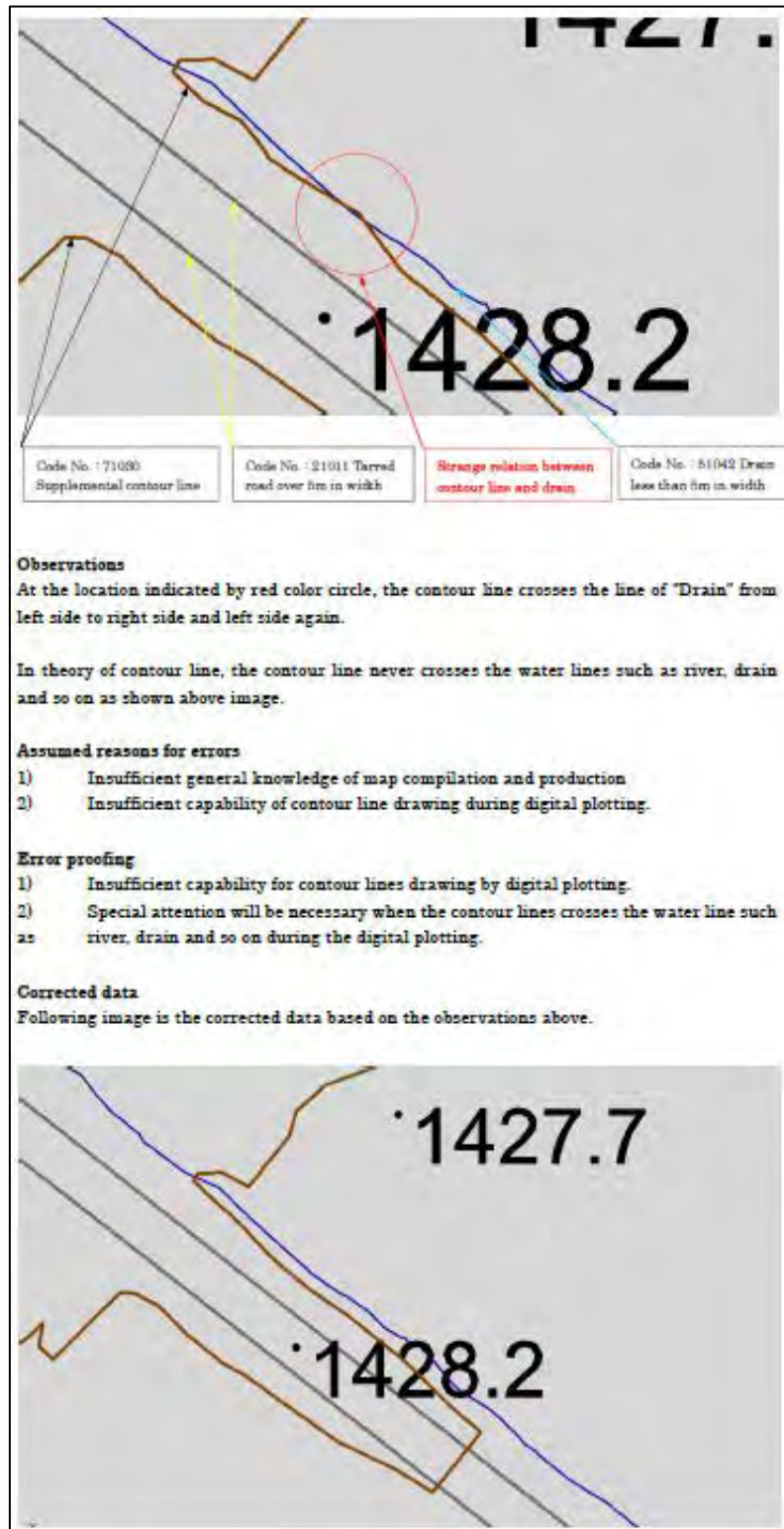
Figure 33 Samples of digital plotting error and countermeasures
