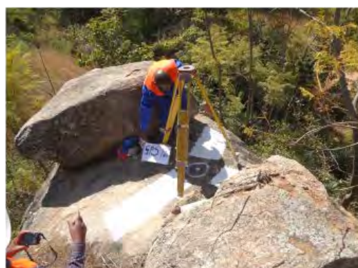
Photo 4 Top-left: Air mark on the road, Top-right: air mark on bare ground. Down-left: air mark on artificial structure, Down-right: air mark on rock.
