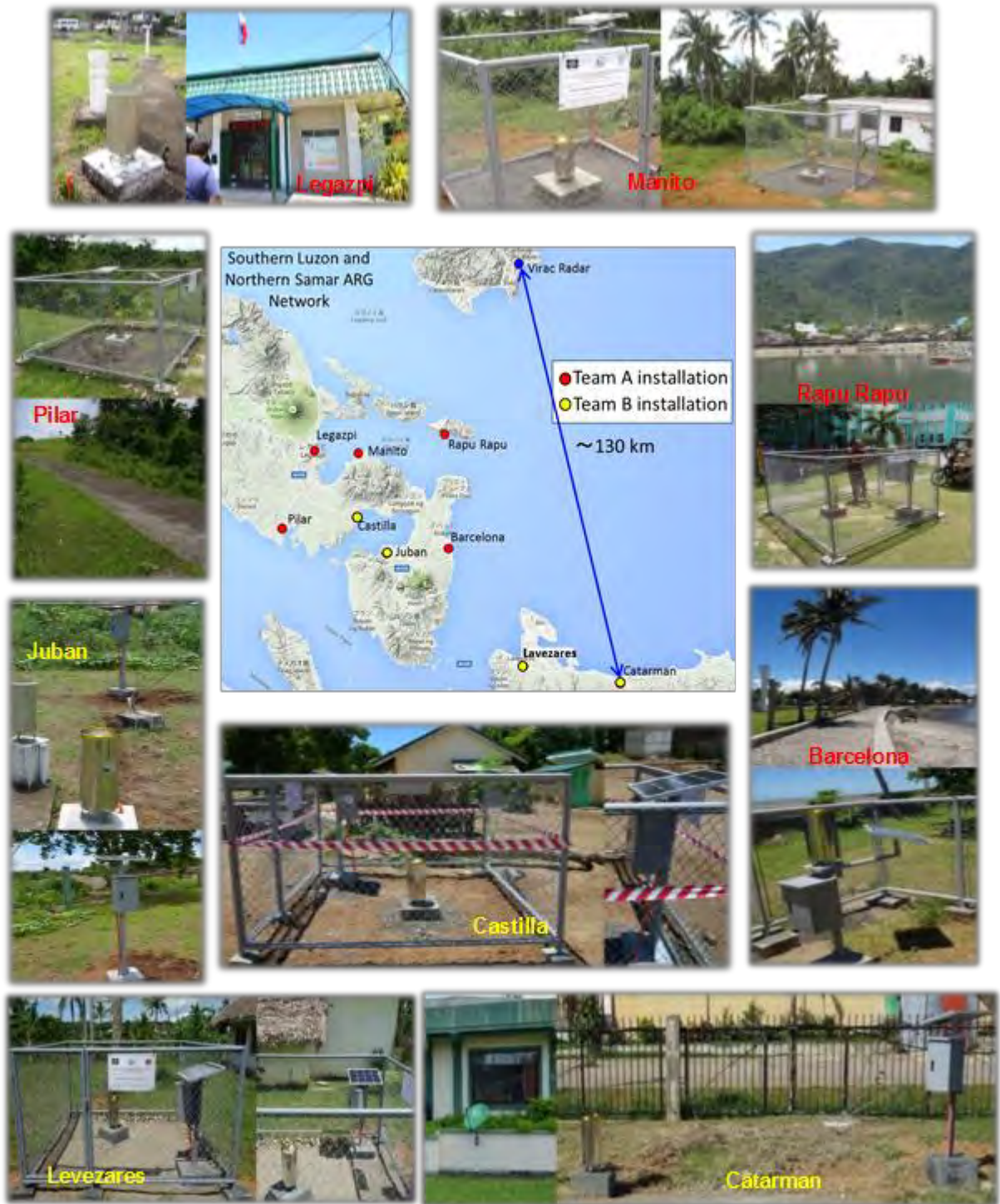
Fig. 3-3-14 Installation sites of the rain gauge observation network in SL-PRSD
