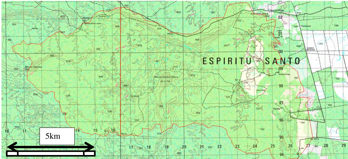
Figure 6-4-1 The Catchment Area of the Sarakata River Hydroelectric Power Plant (Catchment Area=91 km 2 )
