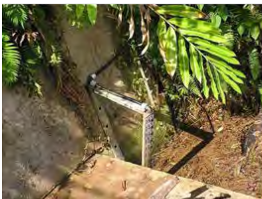
Picture 5-2-3 Water Gauge, Beside Intake Weir.
