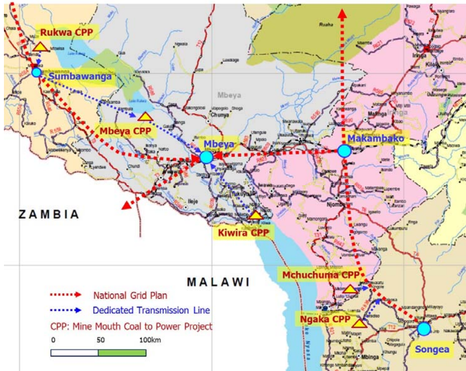
Figure 5.3-2 Mine-mouth Power Plant and Power Transmission Plans
