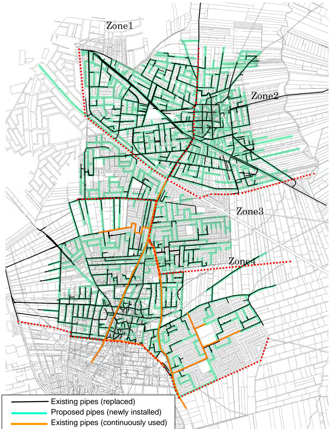
Figure 2.10 Comparison of Proposed New and Replaced Pipe and Existing Pipe to be Utilized
