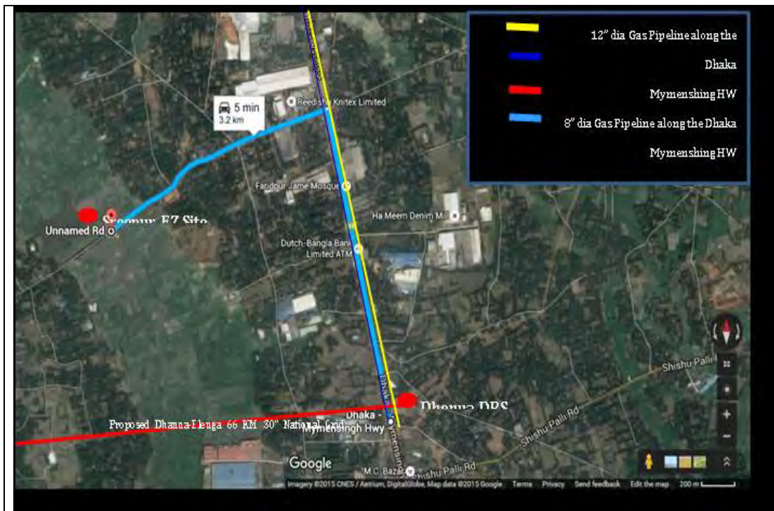
Figure 4.8.3 (5).3 Diagram of Gas Station, replacement tube (light blue), and existing main lines at Nayanpur EZ and Dhonua
