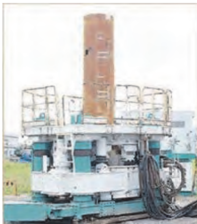
Figure 6.2.5 Photograph of Rotary Penetration Steel Pile (Left: Installation Machine, Right: Tip of Rotary Penetration Steel Pile)
