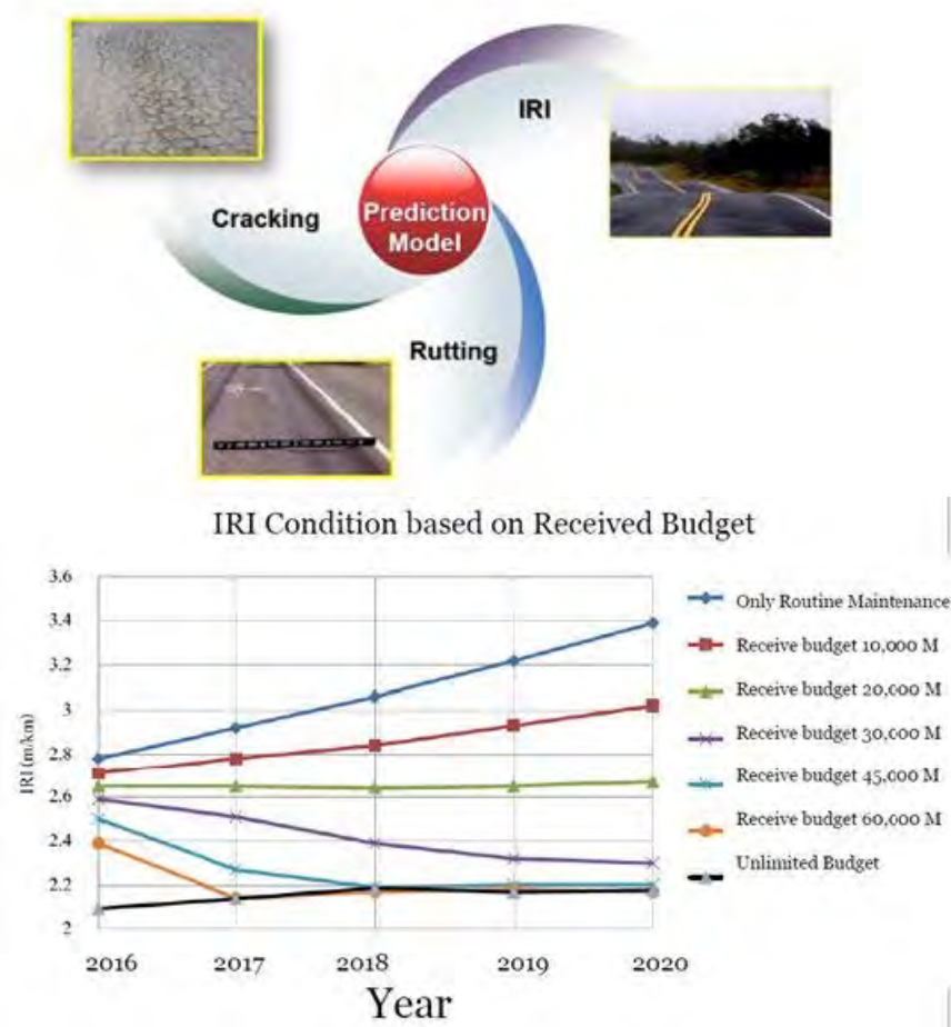
Figure 6.1.8 A case of the technique for introducing a plan to maintain and repair pavements in Thailand
