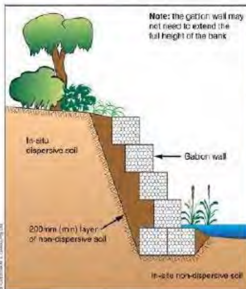
Figure 18 – Gabion stabilisation of gully banks containing dispersive soils
