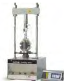
Diagram: mounting equipment for Marshal stability testing (with automatic recorder)
