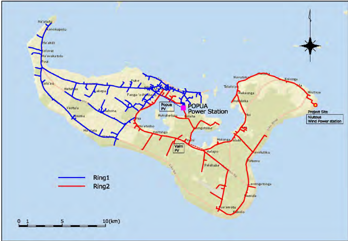
Tongatapu Island, power system diagram (after June, 2017)
