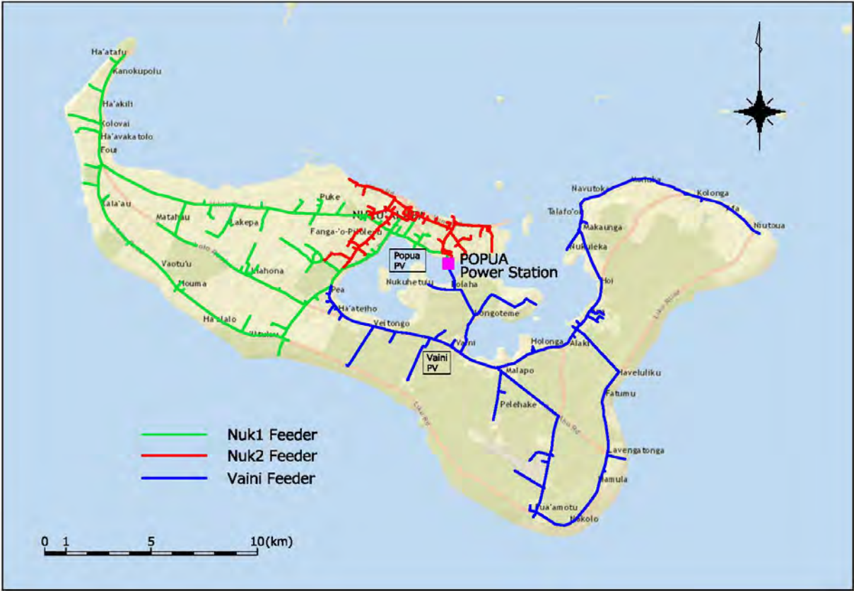
Tongatapu Island, power system diagram (current)
