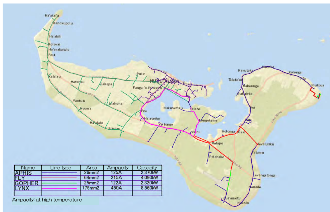
Figure 2-20: Transmission Lines after Expected Enhancement by TPL
