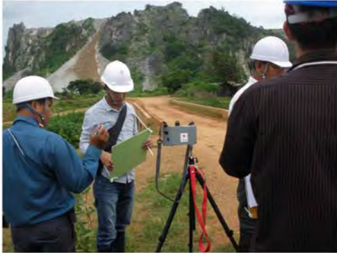
Measurement of environmental dust concentration at near the Limestone mine
