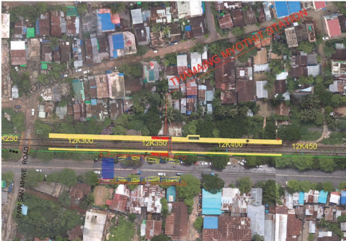
Figure 4.5.27 Proposed Layout Plan and Accessibility (Thrimyaing Station)
