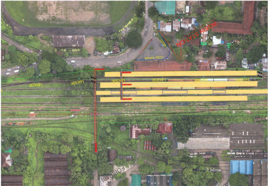
Figure 4.5.43 Proposed Layout Plan and Accessibility (Insein Station)
