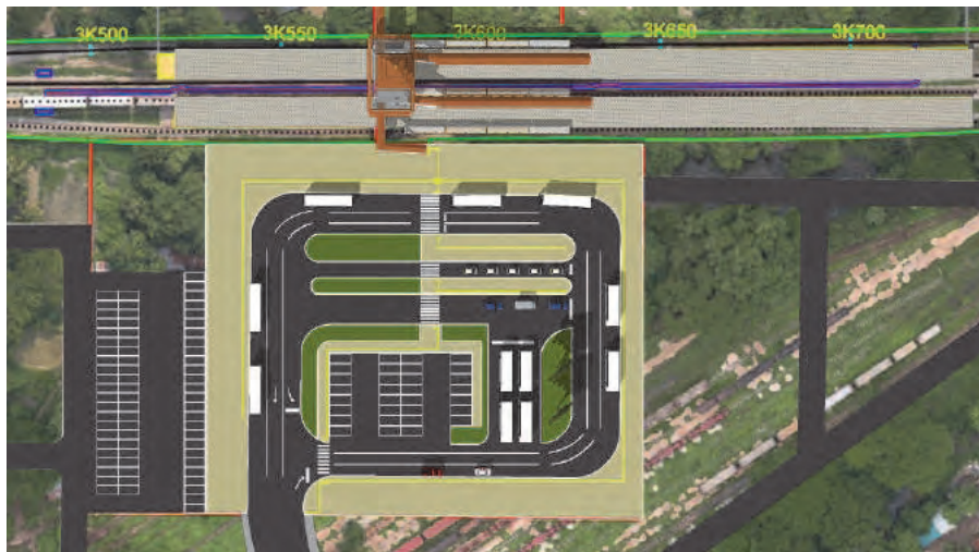
Figure 4.4.8 Layout Plan of the Station Square, Ma Hlwa Gone Station
