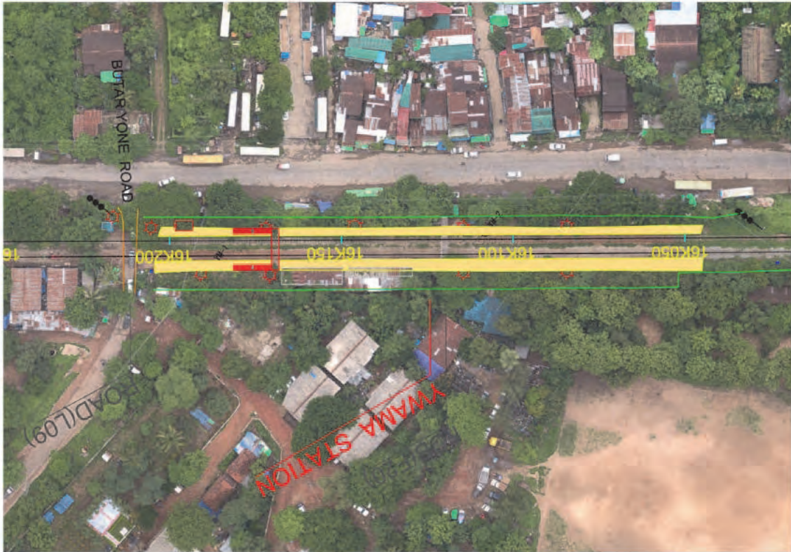
Figure 4.5.35 Proposed Layout Plan and Accessibility (Ywama Station)
