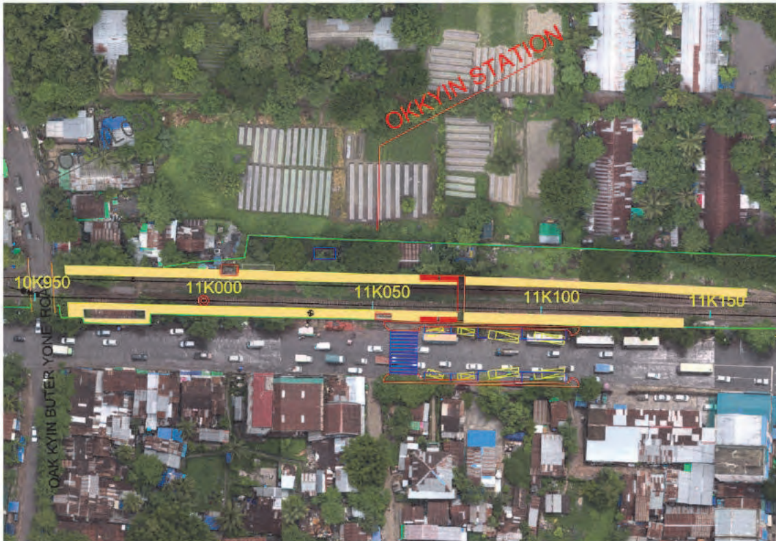
Figure 4.5.29 Proposed Layout Plan and Accessibility (Okkyin Station)
