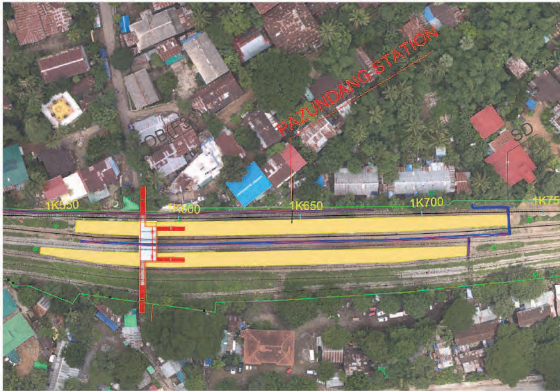
Figure 4.5.13 Proposed Layout Plan and Accessibility (Pa Zun Daung Road Station)
