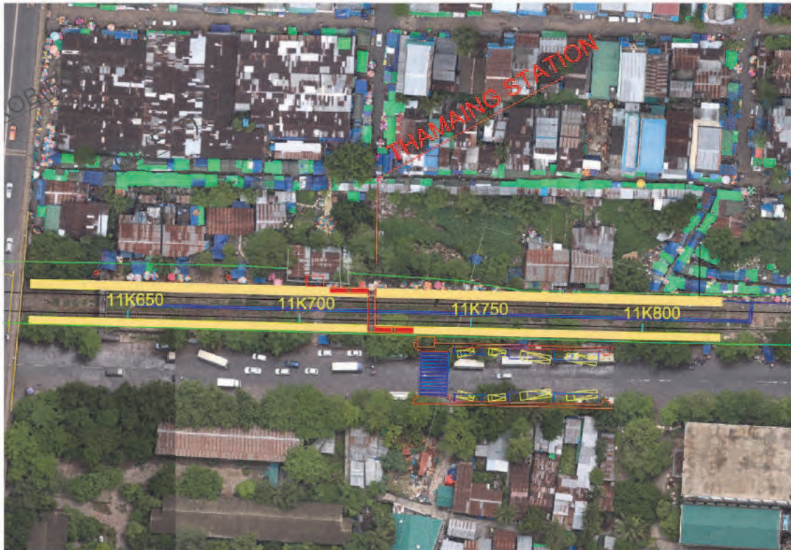
Figure 4.5.11 Proposed Layout Plan and Accessibility (Thamine Station)
