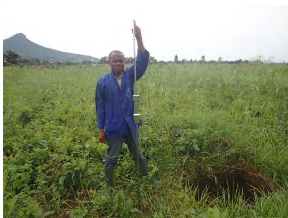
Simple dynamic cone penetration testing
