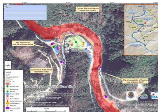
Figure 4.2 Example of Finalized Flood Hazard Map (Bjizam)
