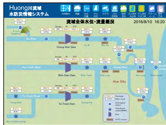
[2] Water level and flow volume of the river, spots where water level is higher than the caution values, dam storage volume figures
