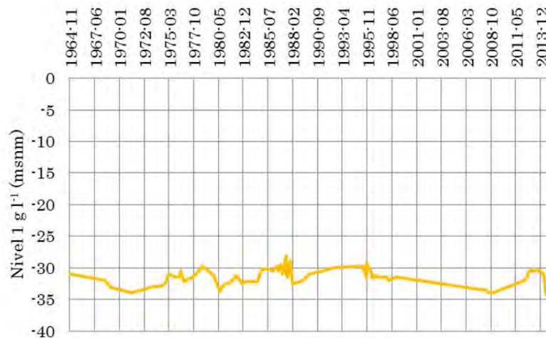
Figure 2-77: Temporal salinity behavior ( 1 \text{ g L}^{-1} ) in the HSC-540 well
