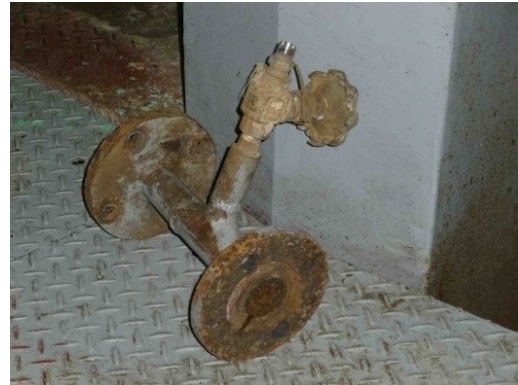
(2) Condition of a small water pipe piece in the turbine pit
