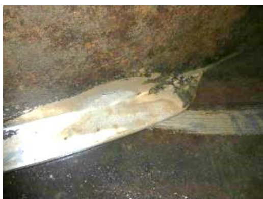
(1) Portions eroded by cavitation
