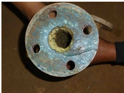
(1) Rust and mud accumulation in the water piping (near strainers)
