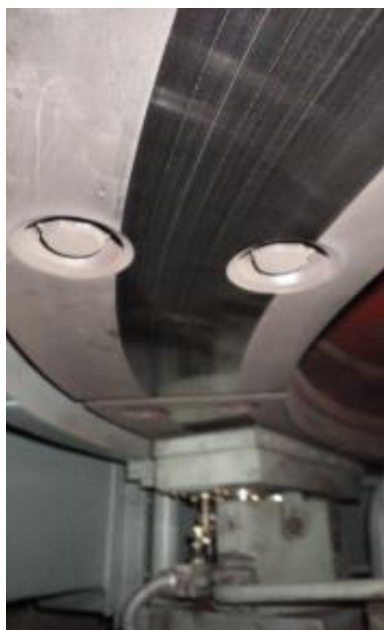
Sliding Scarring of Brake Ring
