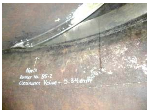
(3) Gap at runner vane periphery
