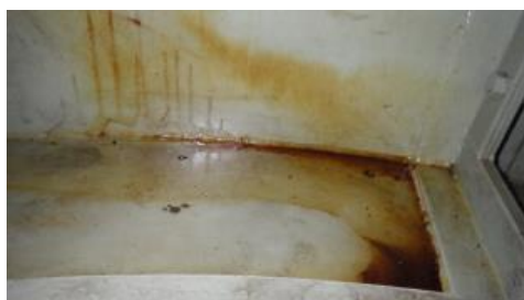
Oil Leakage on Upper Bracket
