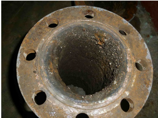
(1) Internal condition of the cooling pipe just after a water pump
