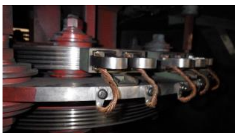
Roughness at Surface of Slip Ring and Carbon Brush Powder
