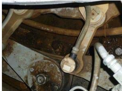
(2) Shear pin breakage detector
