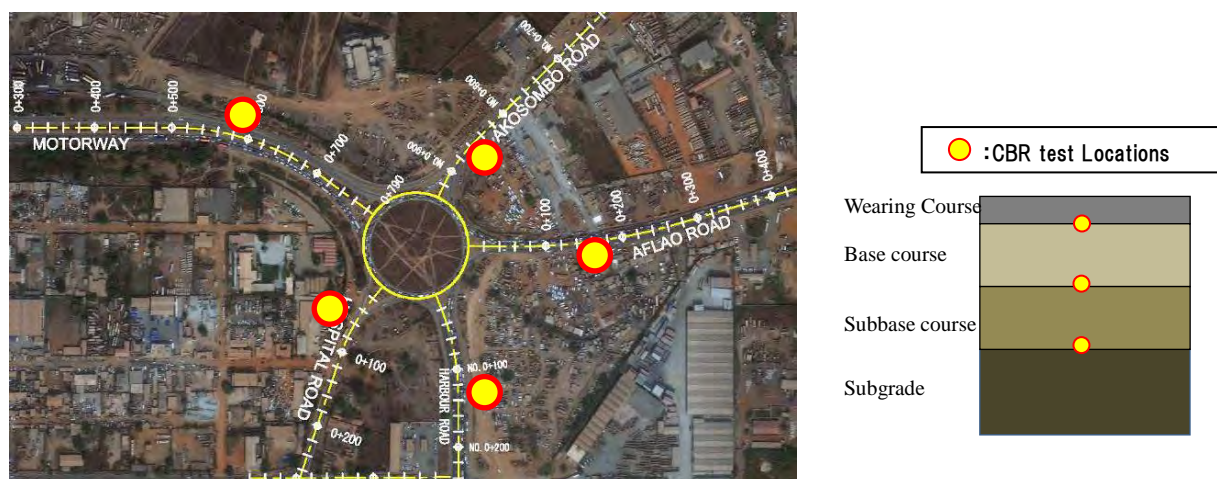
Figure 2.2.2-28 Existing Pavement Survey by Soil Compaction Tester
