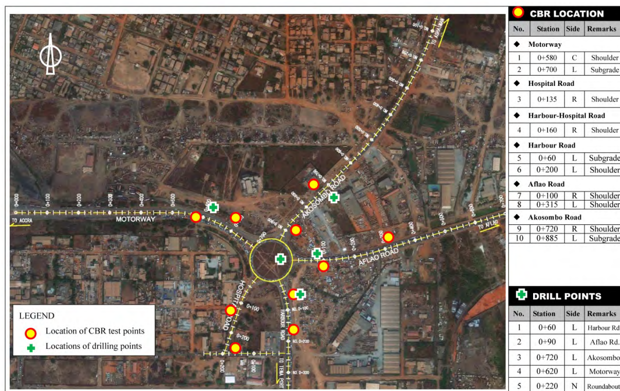
Figure 2.2.1-4 Location of Drilling Points and CBR Test
