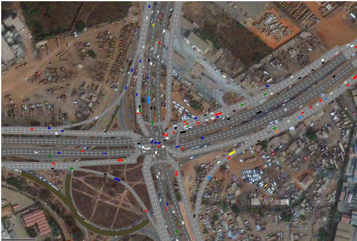
Figure 2.2.2-2 3-tier with At-grade Signal Controlled Intersection (Compact Diamond Type)
