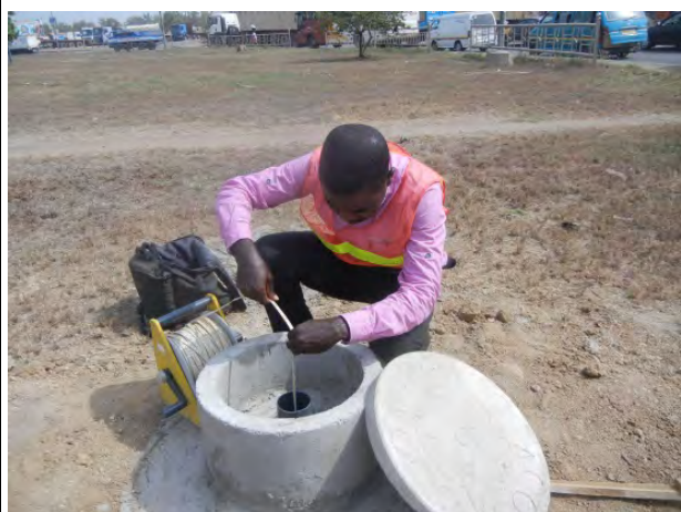
Groundwater level measurement (Observation well)
