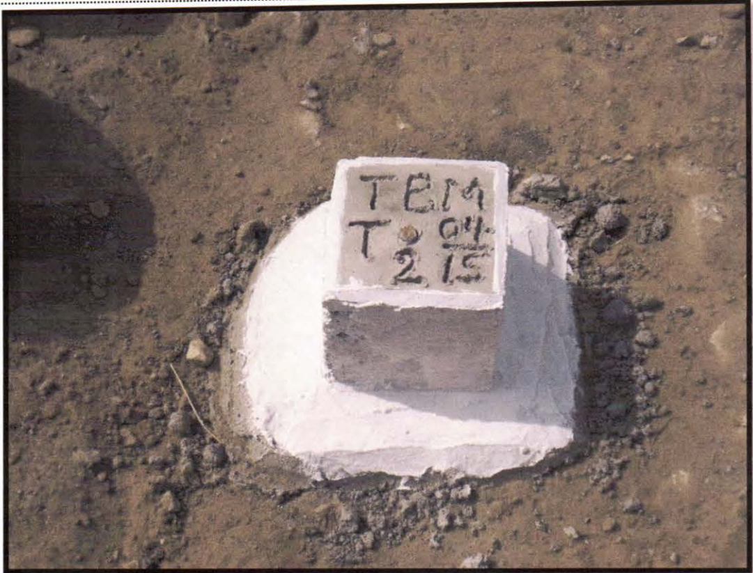
Picture No.9: Temporary Benchmark
