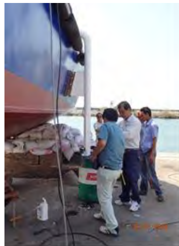
Photo 3 - 8 Survey Boat, PAS Patrol Boat; “KOH DEKKOL”, and Installation of Transducer to the Side Frame of Hull
