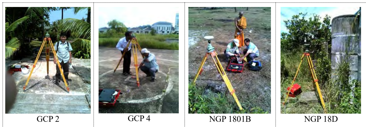
Photo 3 - 2 Control Point Survey by means of GNSS
