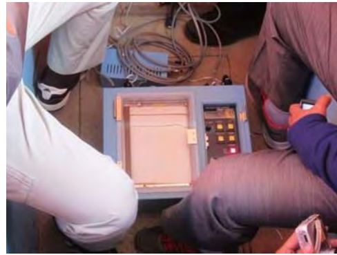
SBES data Acquisition System
