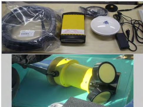
GNSS; SPS351, for Positioning and ADCP,500kHz
