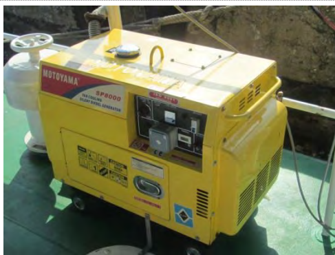
Generator for Survey Boat
