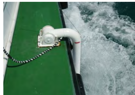
Transducer Cable is in Pipe
