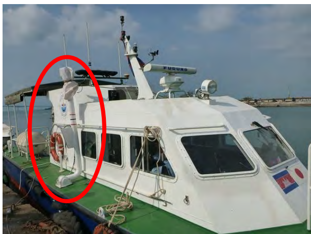
MBES Transducer being raised up when transiting
