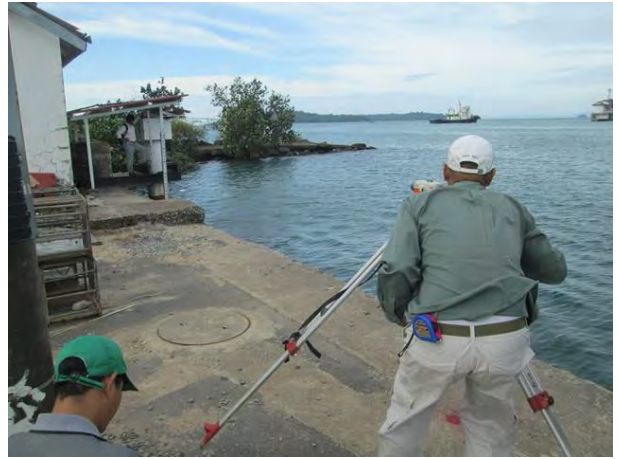
Leveling survey from PAS BM point to Tide Station BM point
