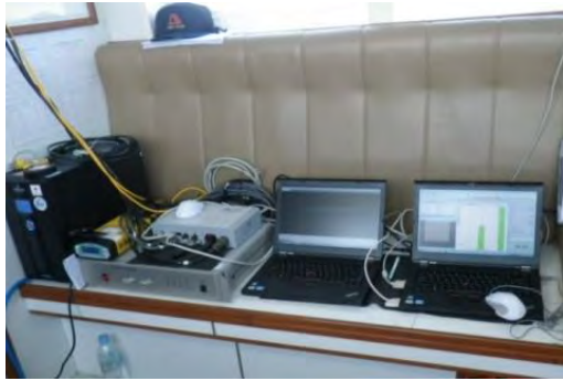
from left: UPS, GNSS receiver (Yellow) and SONIC-SIM, and Junction Box and SONIC control PC, and HYPACK SURVEY PC (Feb. 2014 – Apr. 2014)
