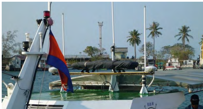
Trimble D-GNSS Twin Antenna at the Roof of Bridge
