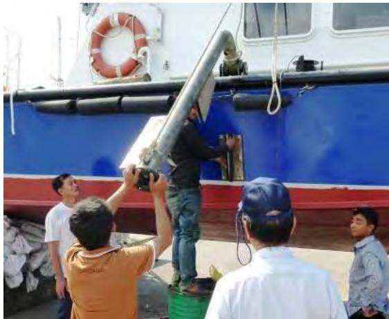
Rigging of Transducer as side-mounted:30 th Jan.2014
