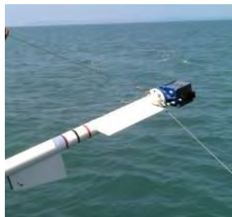
Tip(Blue) is Transducer
