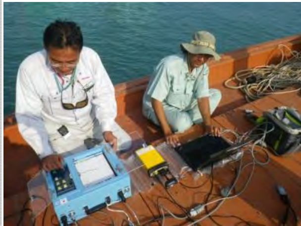
SBES Survey Operation on Board
