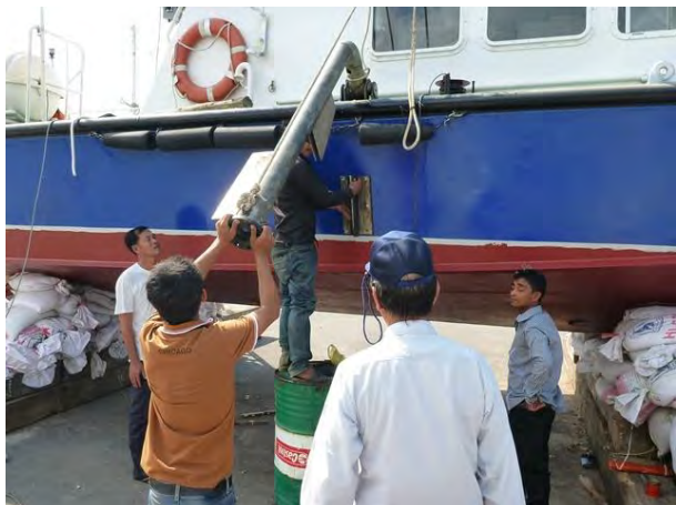
MBES Transducer rigged on to the side frame
