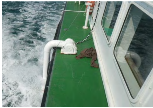
Transducer of MBES mounted with gunwale
