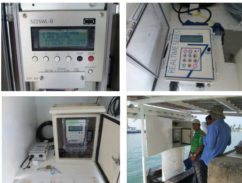
Photo 3 - 14 Comparative Observation of Tides between “RMD5225WL-B” and “RT710”, Simultaneously
