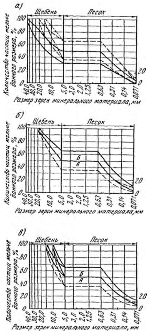
Fig 1.3. Combined Grading of mineral Aggregate : Hot and Warm mixtures with open graded particle size
