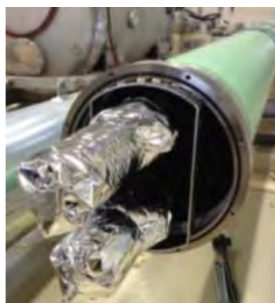
Straight pipe cryostat
