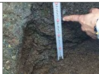
Photo-18 Mix of anthracite and filter sand
