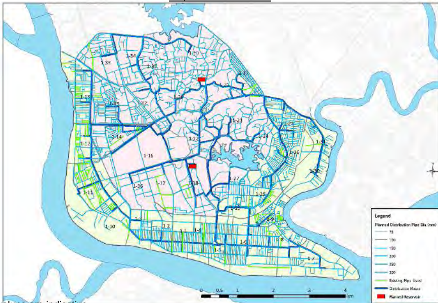
Distribution pipe-network in Zone1
