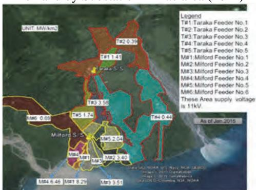
Figure 6.6.4 Electricity Demand Density in Lae area (As of Jan. 2015)
