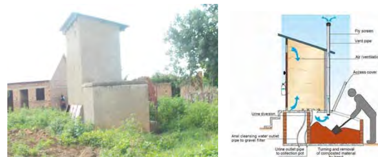
FIGURE 3.06 ECOSAN LATRINE TECHNOLOGY WITH PHOTO OF ECOSAN TOILET NEAR KAMEKE RGC CENTRE
