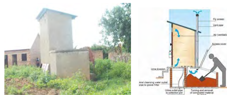
FIGURE 3.06 ECOSAN LATRINE TECHNOLOGY WITH PHOTO OF ECOSAN TOILET NEAR KAMEKE RGC CENTRE
