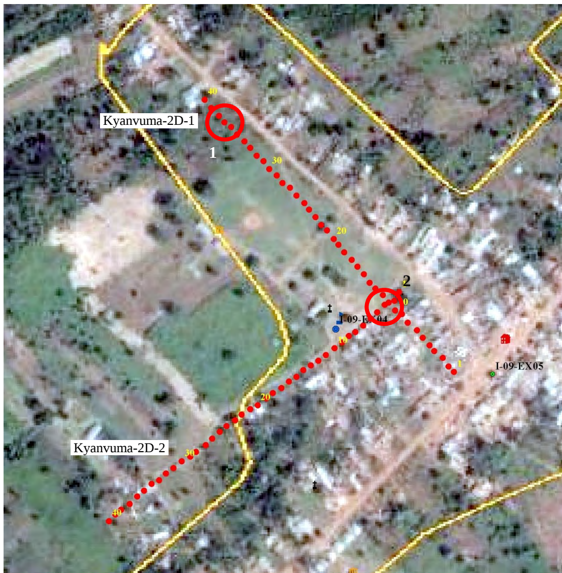
Distribution of 2-Dimensional Resistivity Survey Measurement Line in I-09 Kyanvuma
