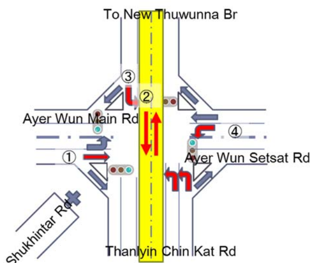
Figure 2-34 Example of Flyover/Underpass to New Thuwunna Rd.
