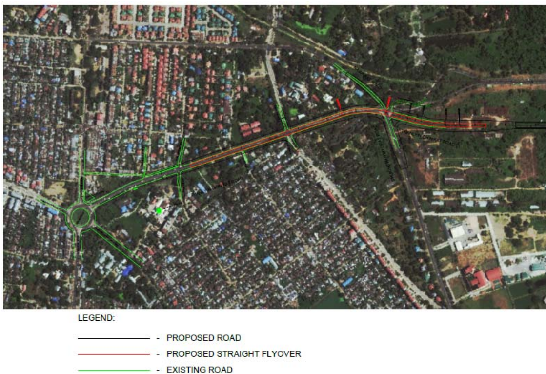
Figure 2: Plan of a straight flyover in Thaketa Township
