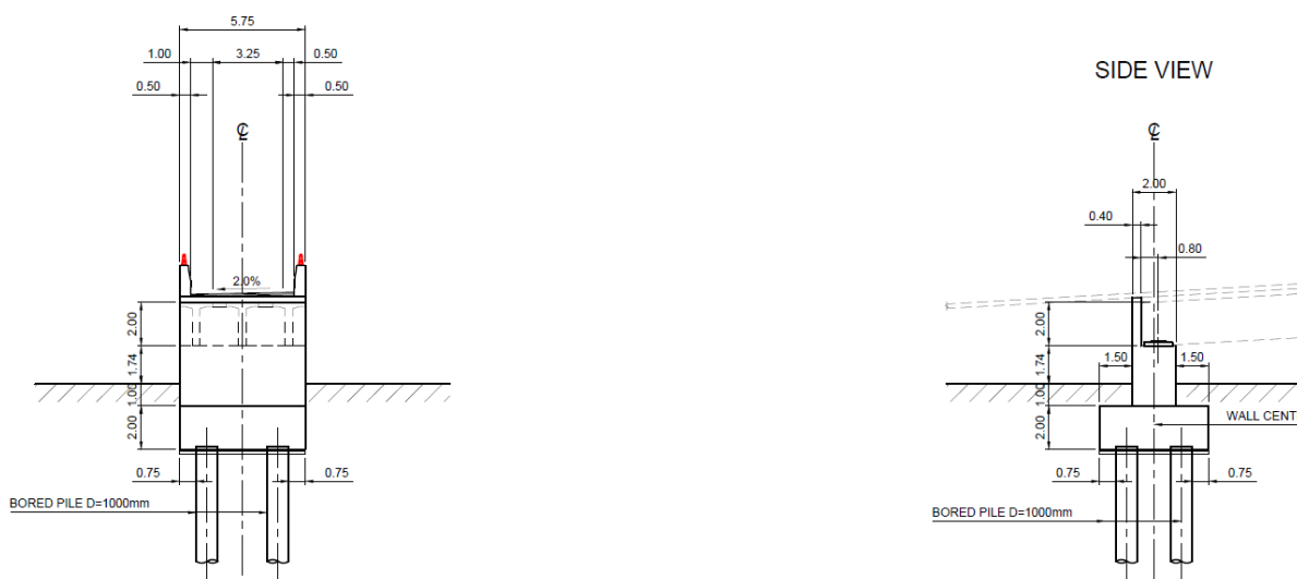
Figure 2-51 Dimensions of Abutment and Height of Embankment
