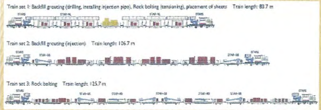
Machine Train Sets for Back Fill Grouting & Rock Bolting
