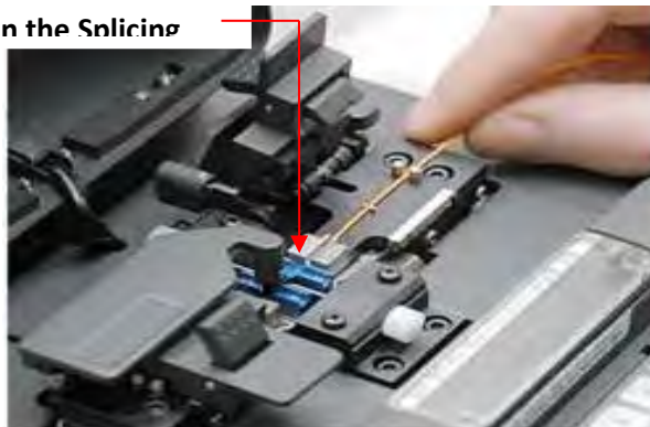
Figure 2-38: Fiber placing on the splicing machine for alignment
