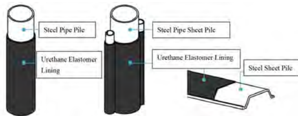
Figure 8.9-3 Heavy-duty Anticorrosion Lining (Urethane Elastomer)
