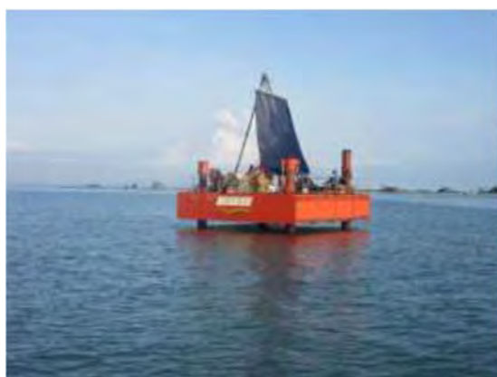
Figure 4.2-2 Boring Jack-up Barge (JUB)
