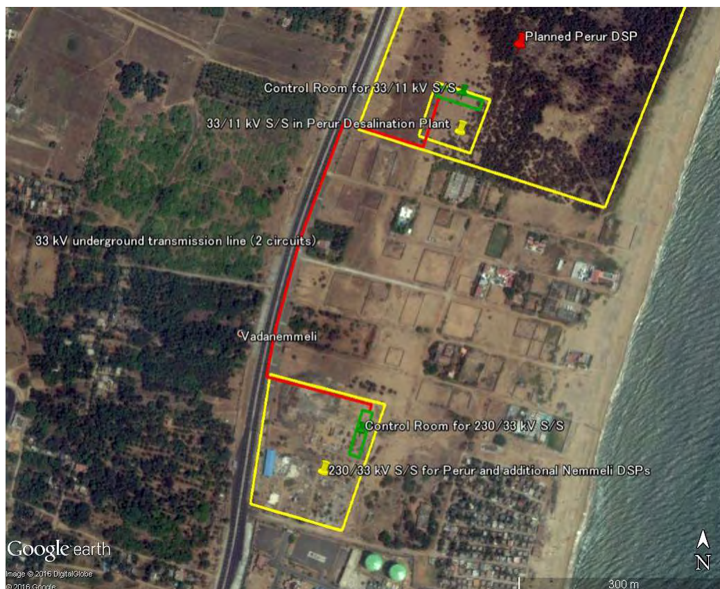
Figure 6.5.3 Power Receiving System for the Perur DSP
