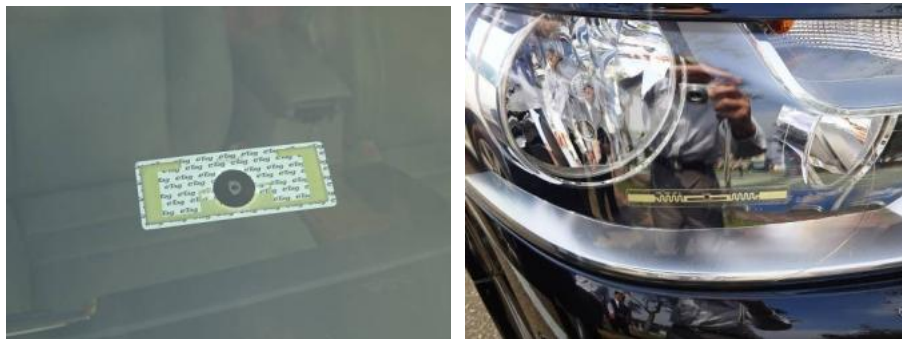
Figure 11.5 RFID Tag Pasted on Windshield and Headlight (for Toll Road Usage) in India
