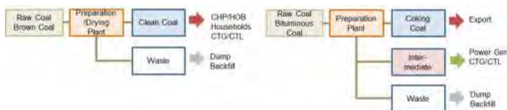
Figure 5.3.2 Preparation Process for Brown Coal and Bituminous Coal
