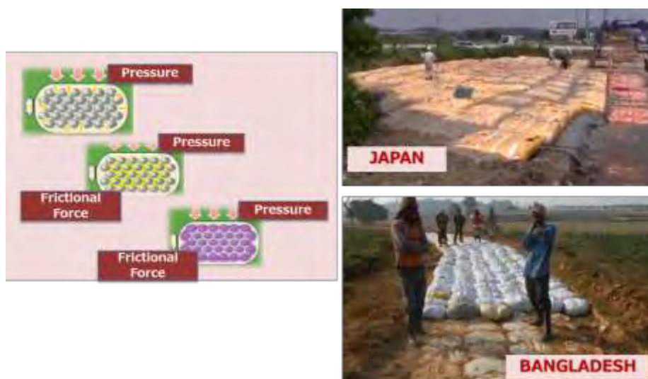
Figure 5.5.1 Concept of Soil Bag Technology and Examples of its Application
