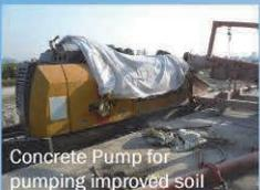
Concrete Pump for pumping improved soil
