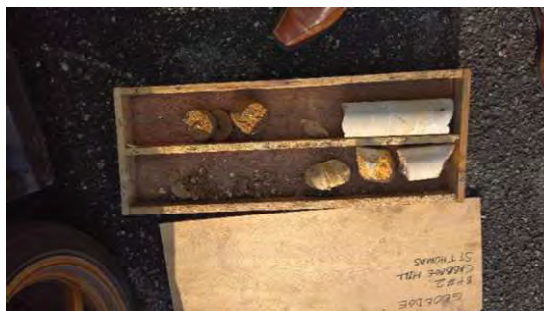
Figure 36 Picture showing core samples collected from borehole, Cabbage Hill, St. Thomas
