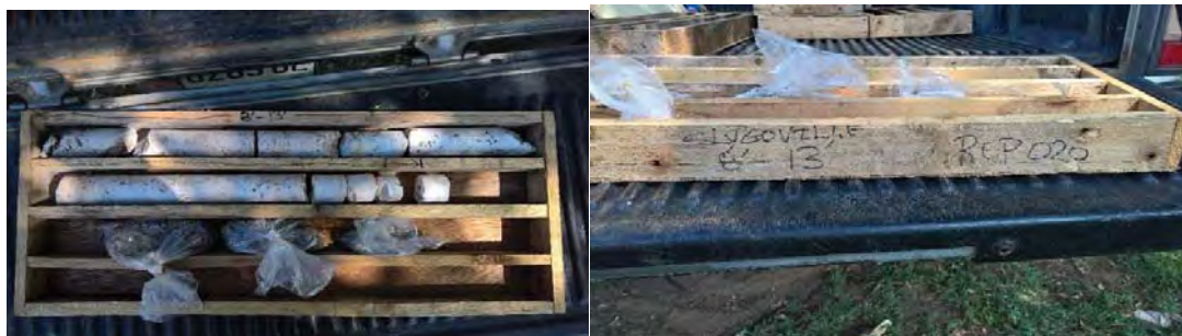
Figure 30 Picture showing core samples from borehole at Sligoville, St. Catherine
