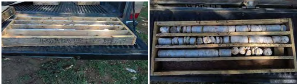
Figure 27 Pictures showing core samples collected from Portland Cottage, Clarendon
