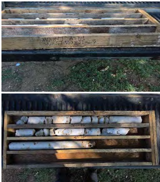
Figure 21 Picture showing core samples collected from borehole, Mt. Airy, Westmoreland
