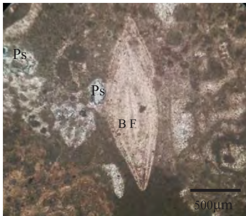
Photo micrograph of sample showing Benthic Forams (BF) within micrite matrix. Pore spaces (Ps) are observed indicated by the blue dye
