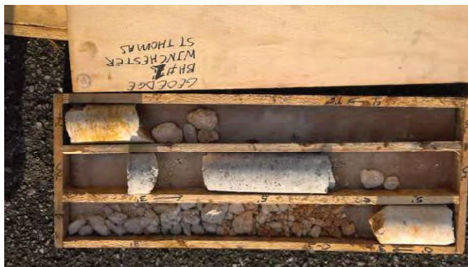
Figure 41 Picture showing core sample collected from borehole, Winchester, St. Thomas
