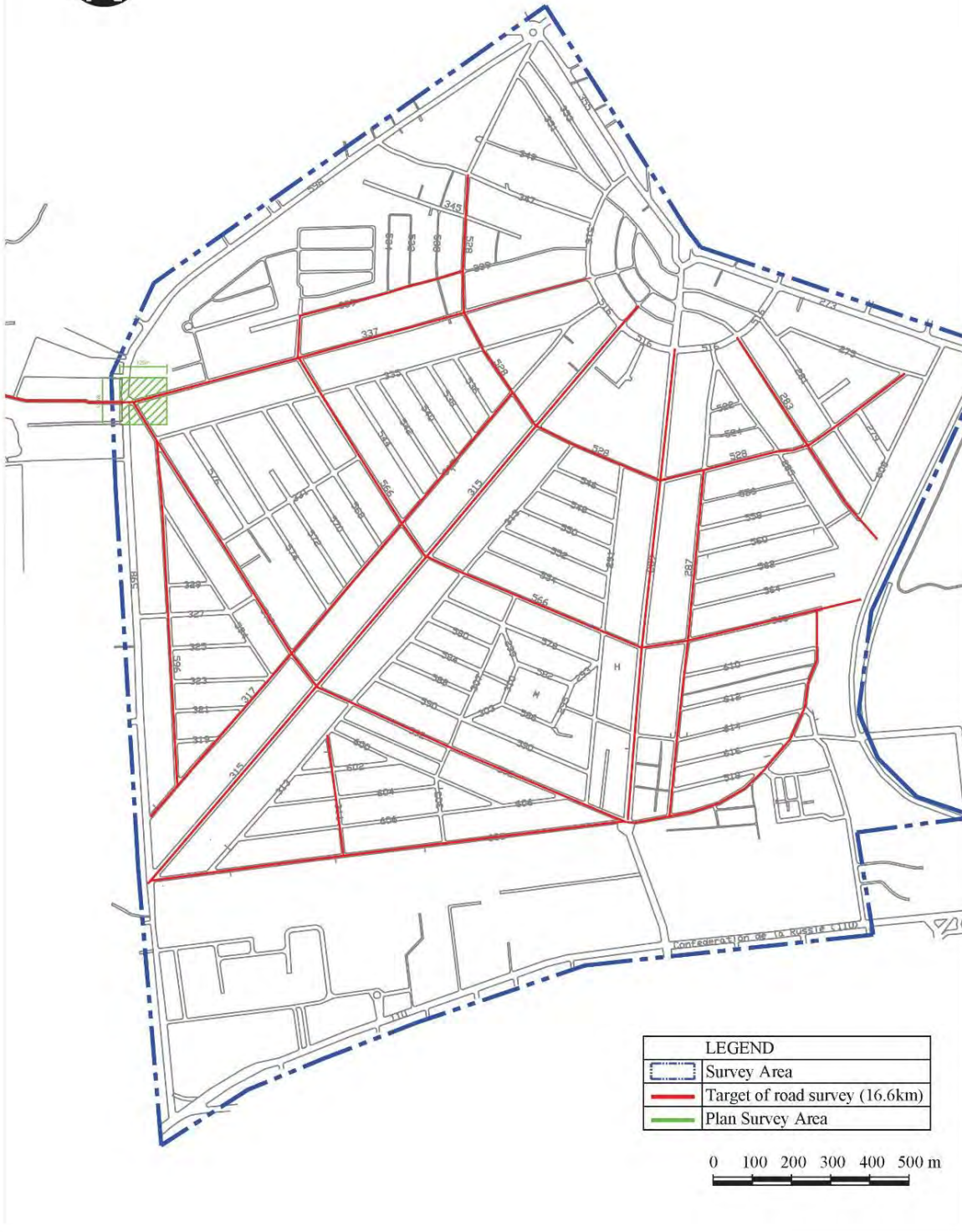
Fig. R 1.3.7 Locations Conducted Topographic Survey (Toul Kork Area)
