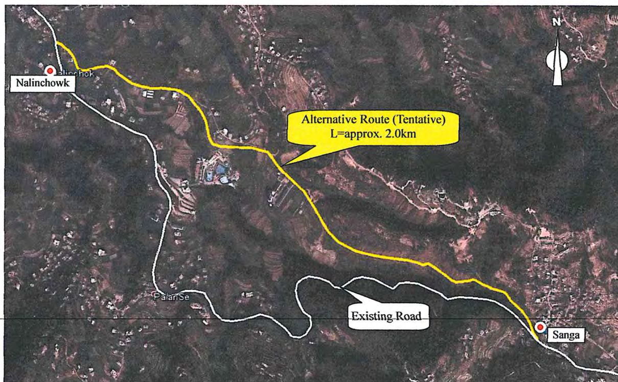
Fig. 2-1 Alternative Route at Mountainous Area
