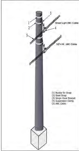
Pole Design of Suspension Concrete Pole 9 Meter for 400 V Line (ABC Cable)
