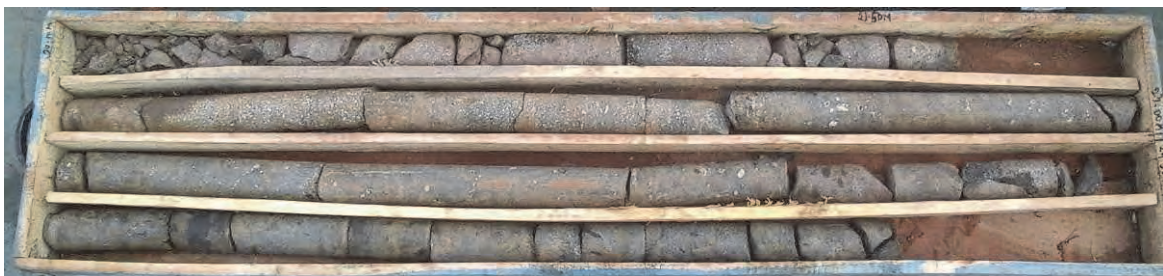
Figure 5.2.3 Core Photo of Basalt Rock
