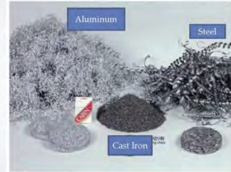
Processing chips of Iron and Aluminum
