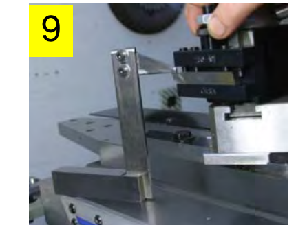
9 Tool centre height adjustment jig
