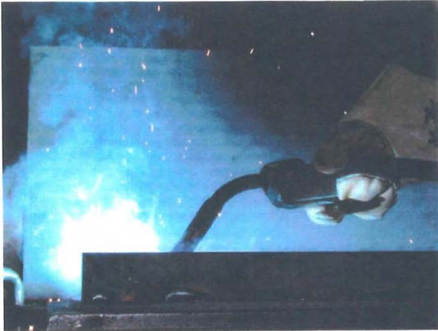
Flux-cored wire (300A,33V)
